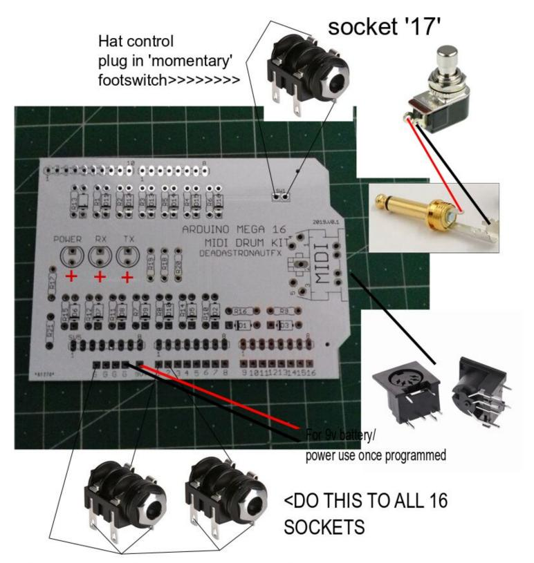
When nothing is plugged In socket tip is sent to ground
